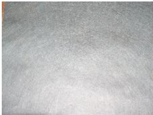
Fig. 3: Copper + nickel plated non-woven polyamide fabric.
