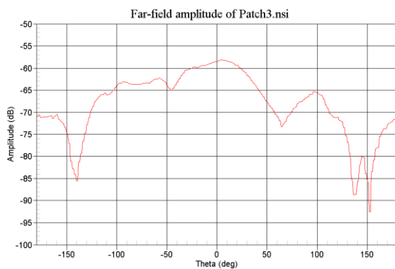
Fig. 11: Non normalized far field radiation pattern for Betex (E-plane).
